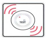
Smoke alarms should be tested once a month by pressing the TEST button.
